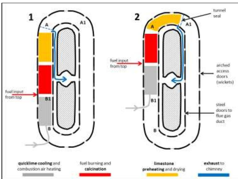
*Plan view of Hoffmann kiln showing principle of operation. The zones are located inside an annular tunnel. The exhaust gases leave via a chimney located above the central blue arrows on the diagram.*
